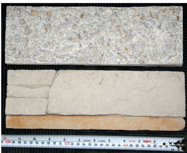
Rear and front face views of the stackstone cladding. The pebbles of pumice can be seen in the cementitious matrix.
