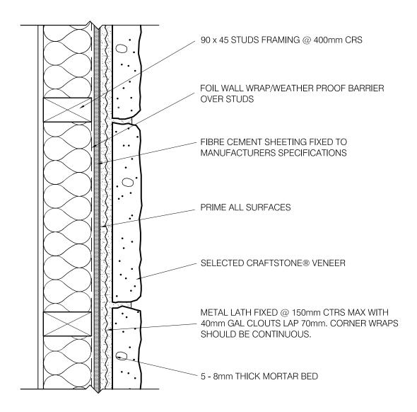
CRAFTSTONE®- FIBRE CEMENT CLAD PLAN DETAIL
